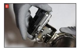
A) Remove the electronic actuator from the original exhaust.
